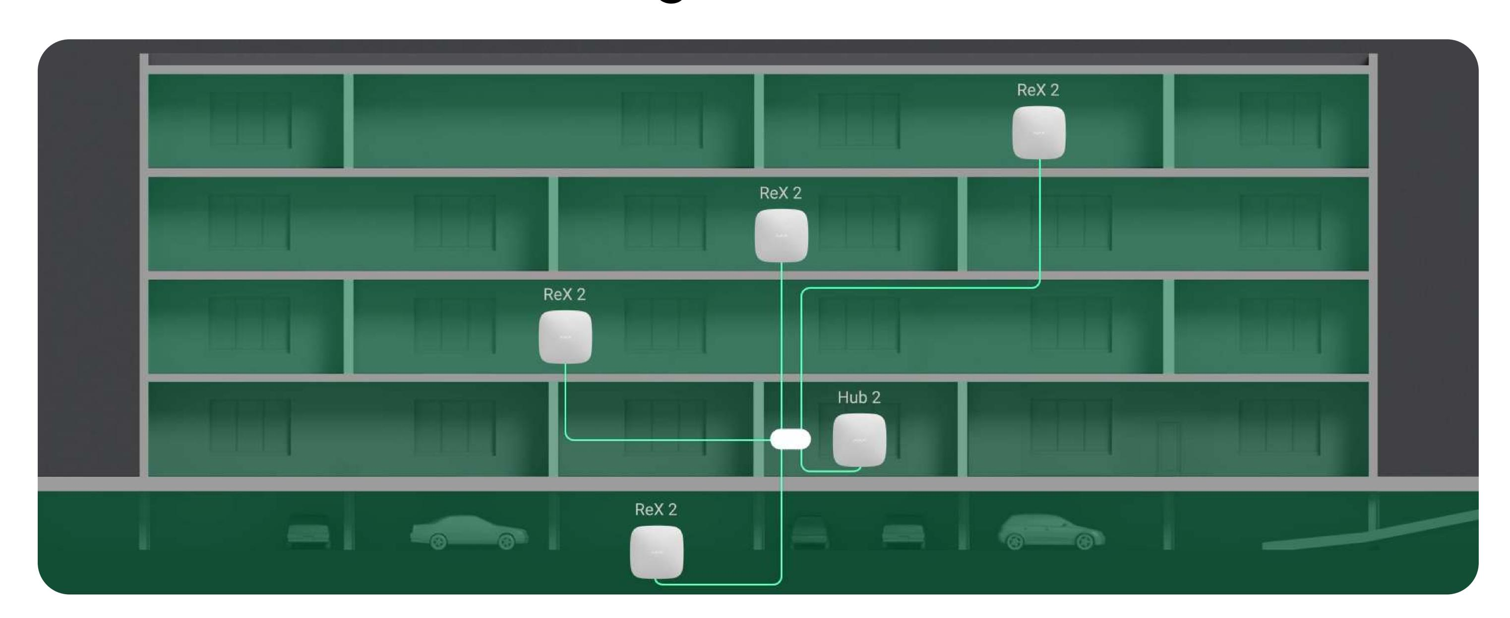
ReX 2 with **OS Malevich 2.13** firmware transmits data to the hub via radio and Ethernet cable. The cable can be used as the only or additional communication channel. The hub and the range extender must be connected to the same network through a router for that. An Ajax security system does not limit the length of the cable. Thus, one system can cover such an object as an office center with underground parking, a metal sectional hangar or a warehouse complex of several buildings.
