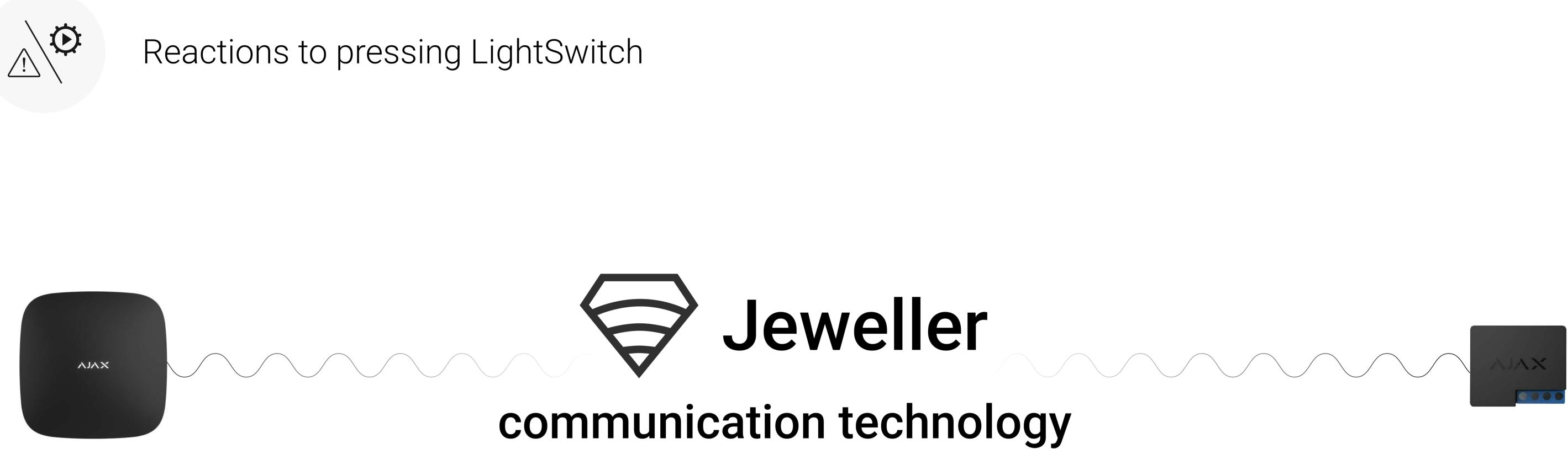
Jeweller is a wireless data transfer protocol to provide fast and reliable two-way communication between the hub and connected devices. The protocol helps monitor and control connected devices via Ajax apps. All data transfers – from the hub to a device or the cloud – are delivered in small data packets and protected with floating key encryption.
