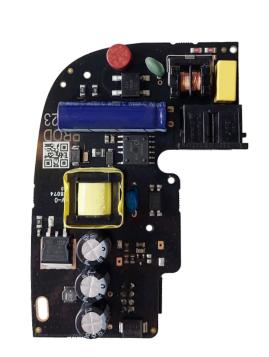
220V PSU for Hub/Hub 2/Hub 2 Plus/ ReX 2 Control panels
